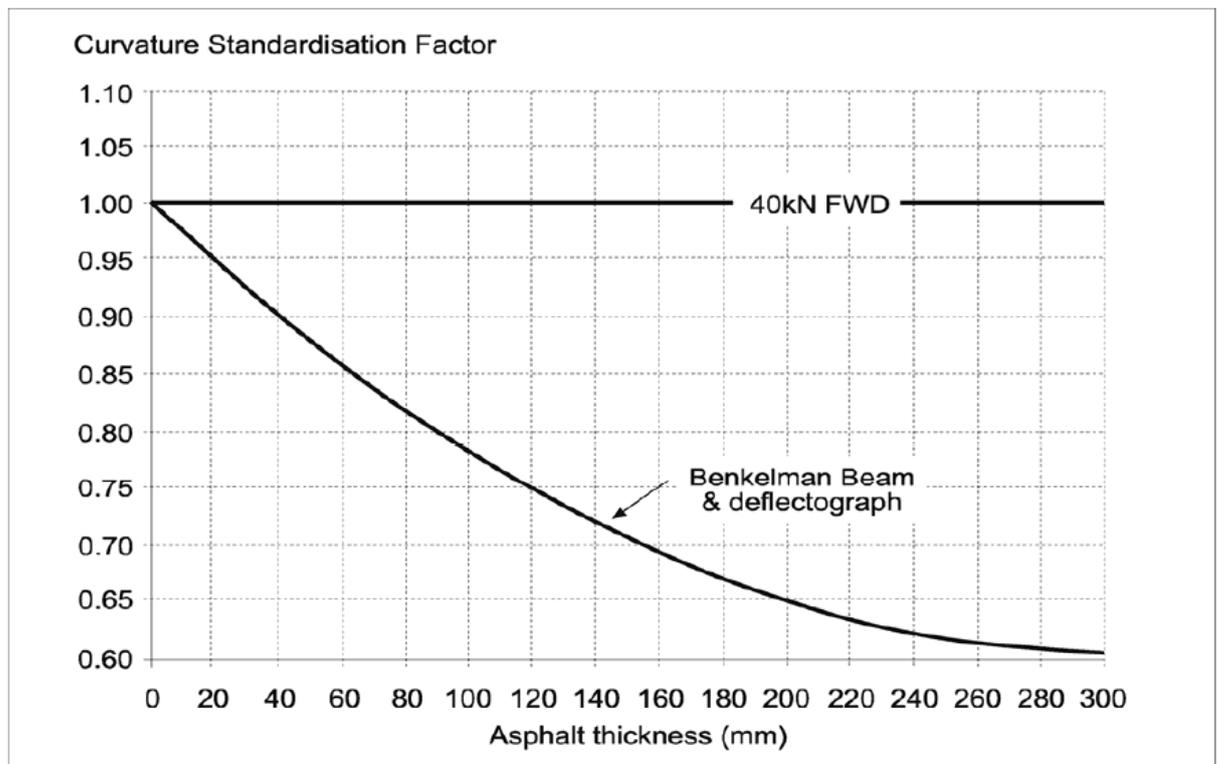
Figure 6.4: Curvature standardisation factors
