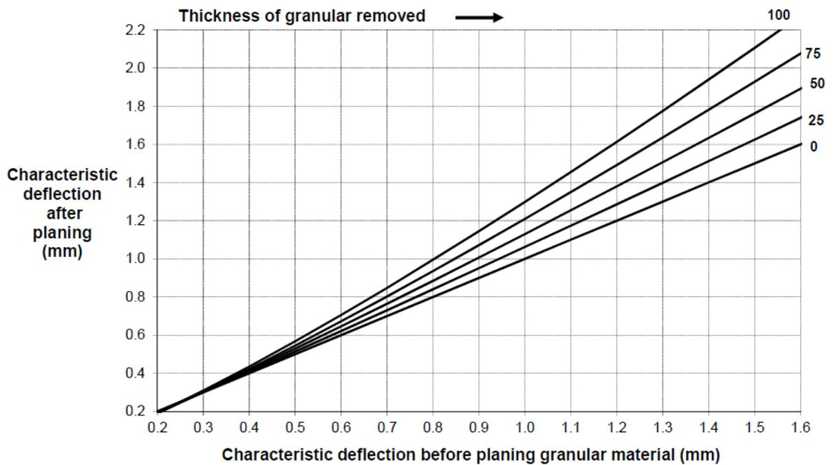
Figure RD-PV-D2 7-6 Increase in curvature due to removal of granular material
