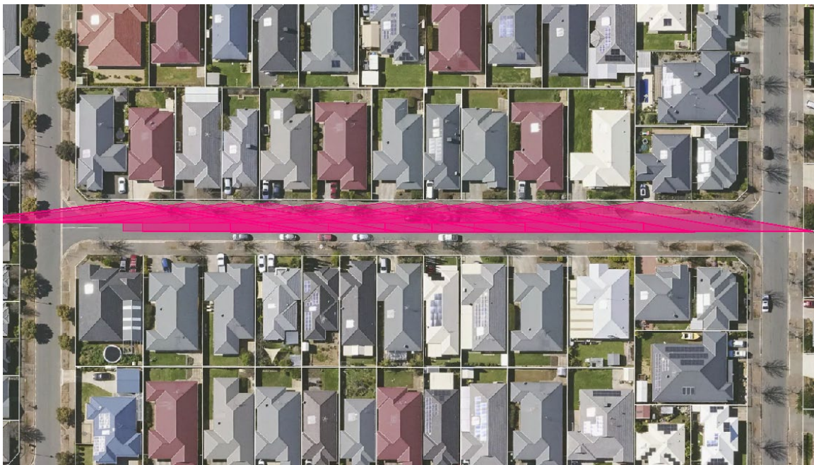
Figure 1 - Overlay of 45m sight line triangles for each crossover on just one-side of a road
