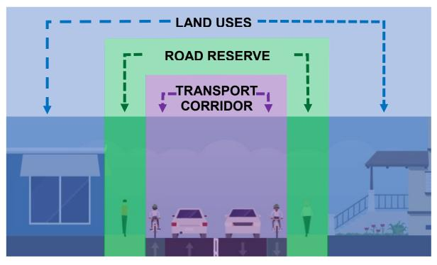
Figure 18: Typical cross section of a road-based transport corridor. Source: InfraPlan
