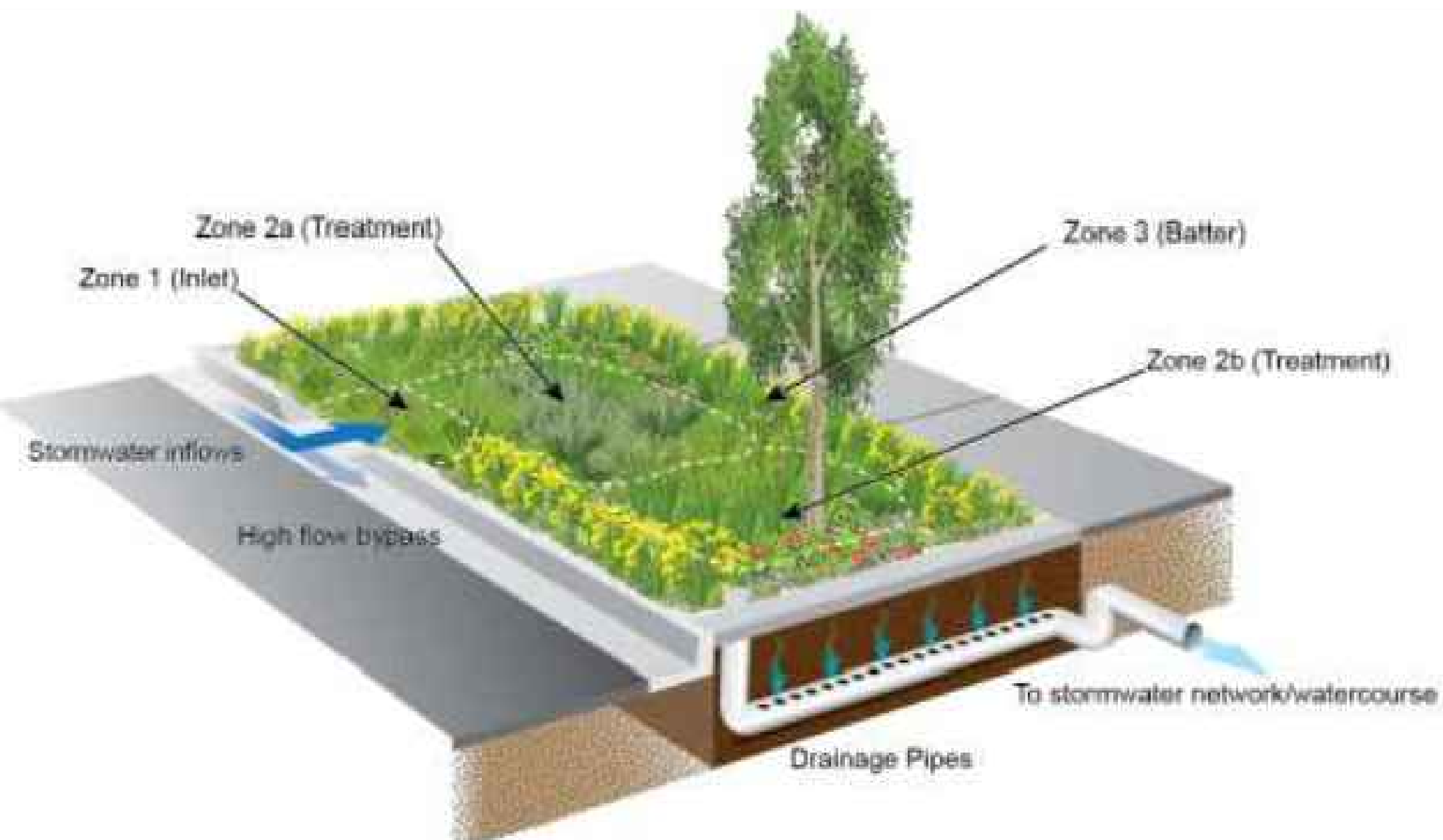
TYPICAL KERB SIDE RAINGARDEN BIO-FILTRATION LAYOUT
