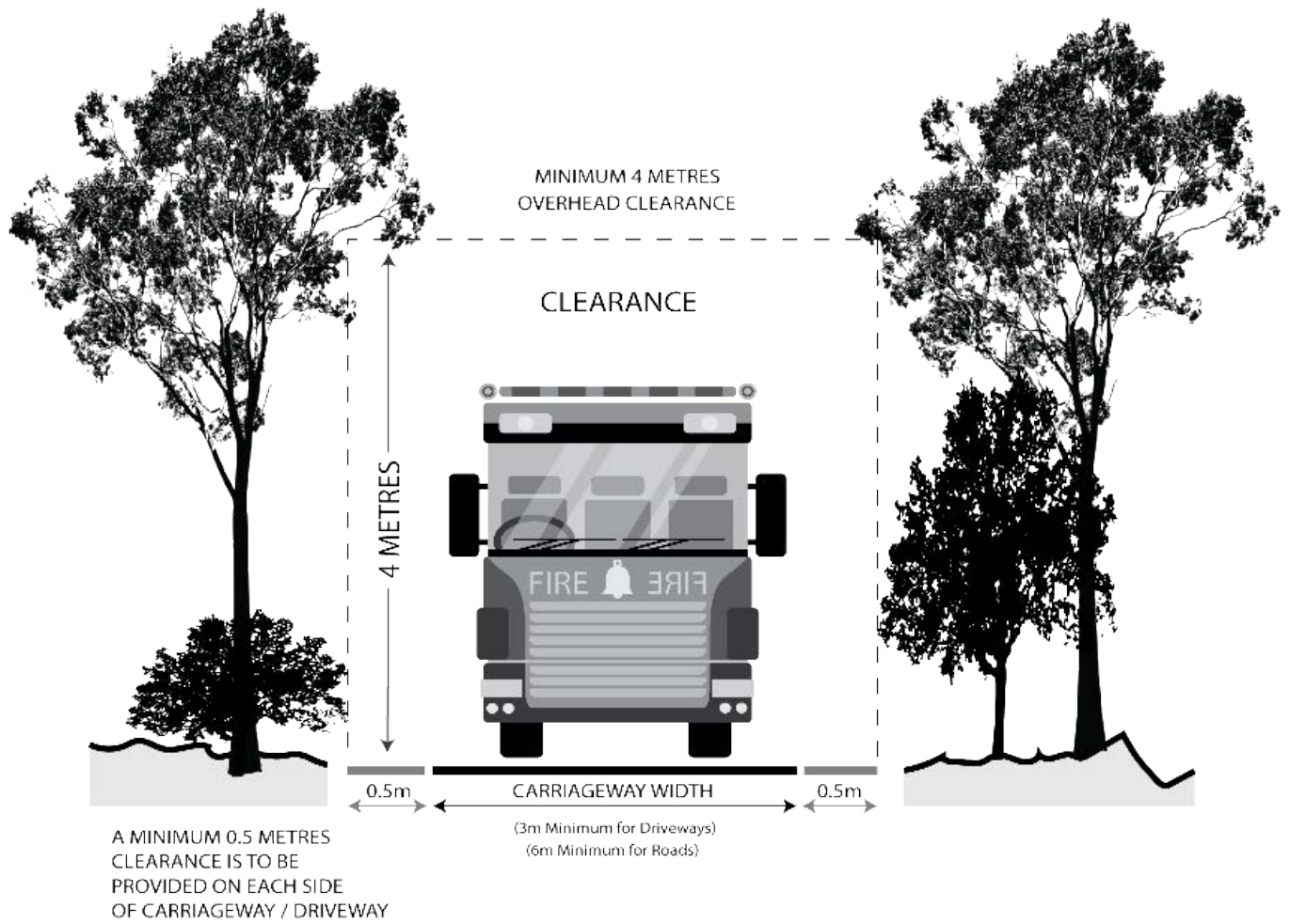
Figure 1 - Overhead and Side Clearances
