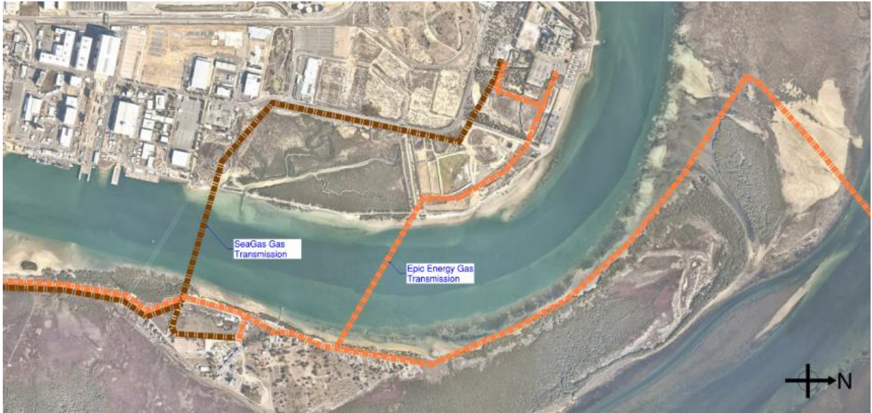
Figure 8 – Epic Energy and SEA Gas high-pressure gas pipelines
