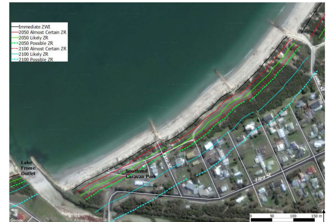
Figure 5: Potential Extent of Erosion in Southend
