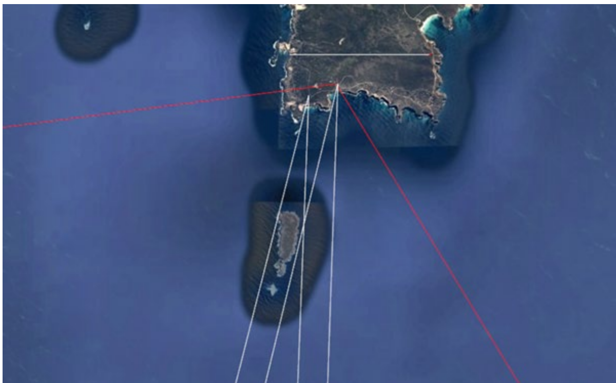
Figure 9. Range of possible bearings for sun synchronous and polar trajectories from each launch site. Source: Southern Launch (see Appendix 1).
