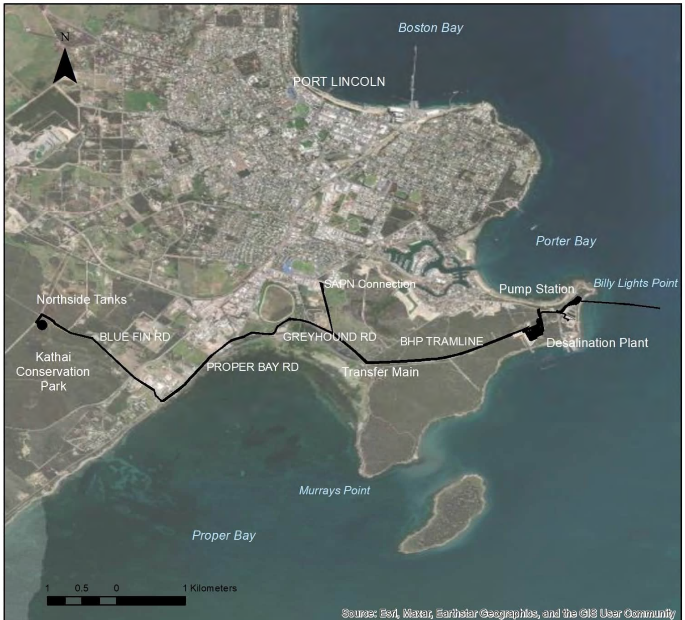
Figure 3. Desalinated water, Saline Waste/Seawater Transfer mains including SAPN connection footprint which will require removal of Native Vegetation.
