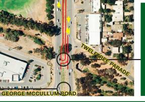
A new sheltered u-turn lane has been installed, operating one way for southbound drivers. Twelftree Parade remains left in and left out only.
