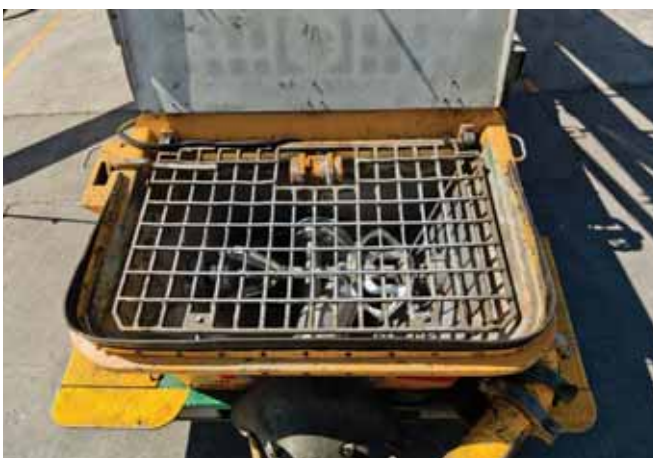
Hopper safety grill - double bar
