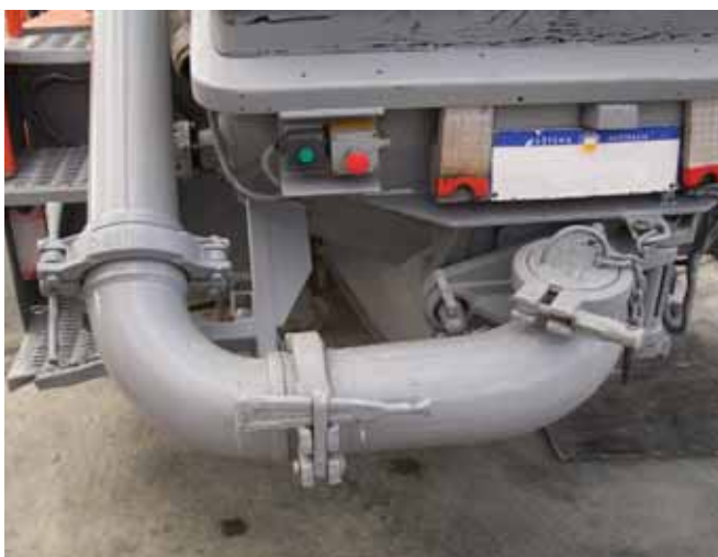
Concrete pipe with safety pins
