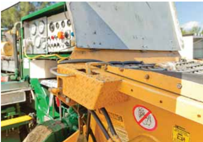
Interlocking mechanism which shuts down the pump if the grate is lifted
