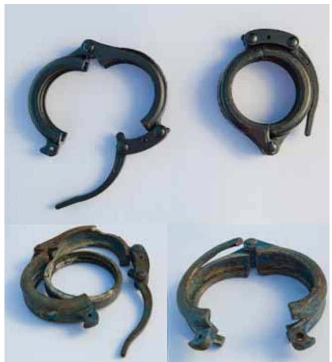
New and damaged pipe clamps
