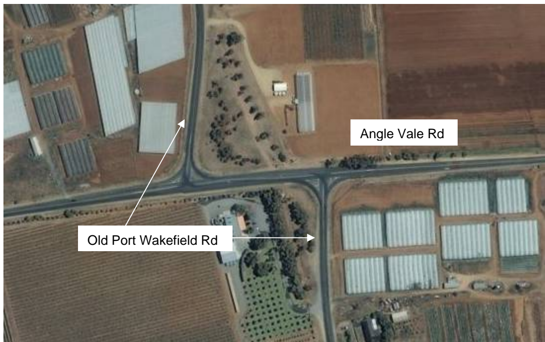
FIGURE 5.3 Existing staggered T intersection of Old Port Wakefield Road at Angle Vale Road
