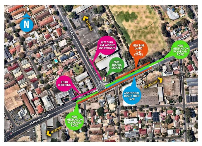
The map below shows the design features of the new road configuration and junction upgrade.
