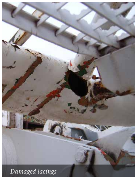
Initial damage to the carousal when lowering the boom to the ground
