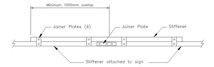
A minimum overhanging length of 1000 mm is required for the stiffeners at vertical joins.
