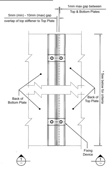
NOTE : \* = > 2000 use a minimum of 3 Fixing Devices < 2000 use 2 Fixing Devices
