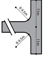
"T" shaped turning area for fire trucks to reverse into so they can turn around
