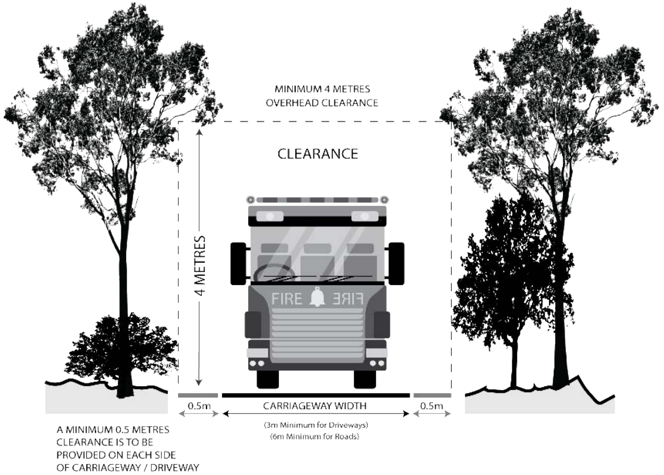
Figure 1 - Overhead and Side Clearances
