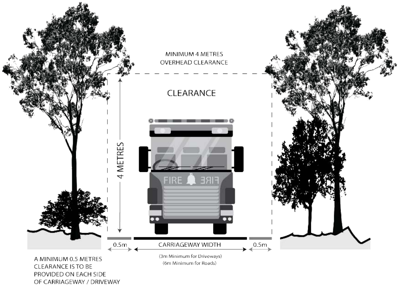
Figure 1 - Overhead and Side Clearances
