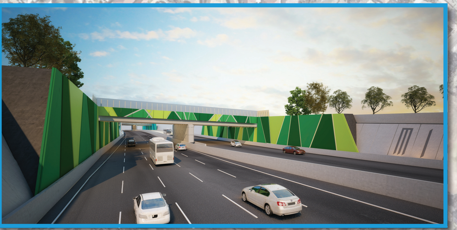
Artists impression of lowered motorway and Sturt Road bridge including throw screens and coloured panels for wayfinding.
