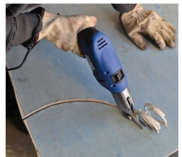
Shears can be used instead of cutting (when practicable)
