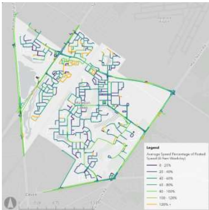
Figure 7: Average speed as percentage of posted speed limit during weekday AM Peak (8-9am)
