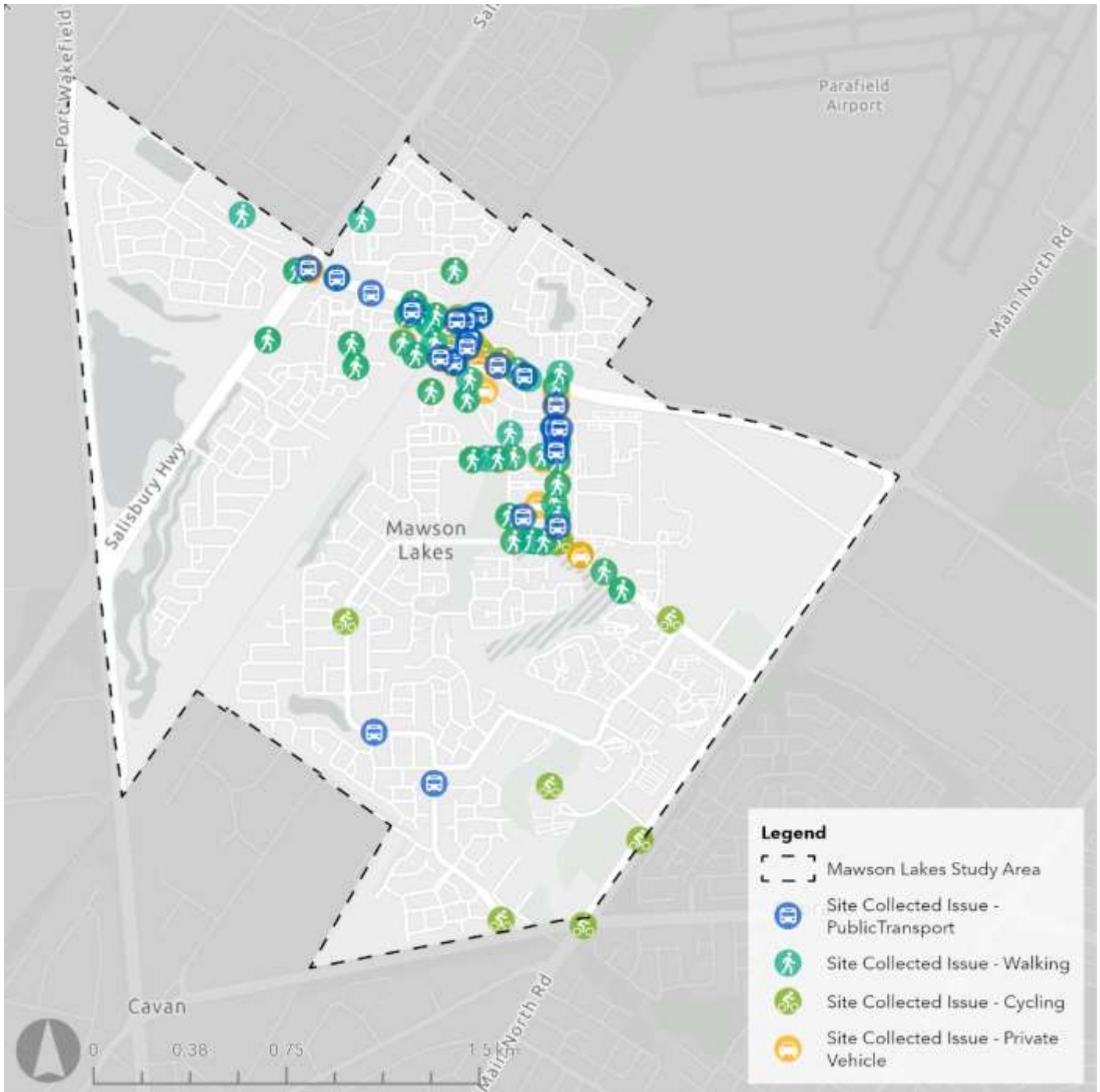
Figure 3: Site Investigations – mode issues identified
