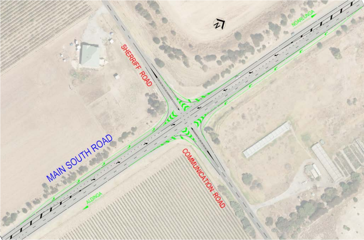
Figure 6-6 Proposed Upgrades for Main South Road/ Sheriff Road/ Communication Road Intersection
