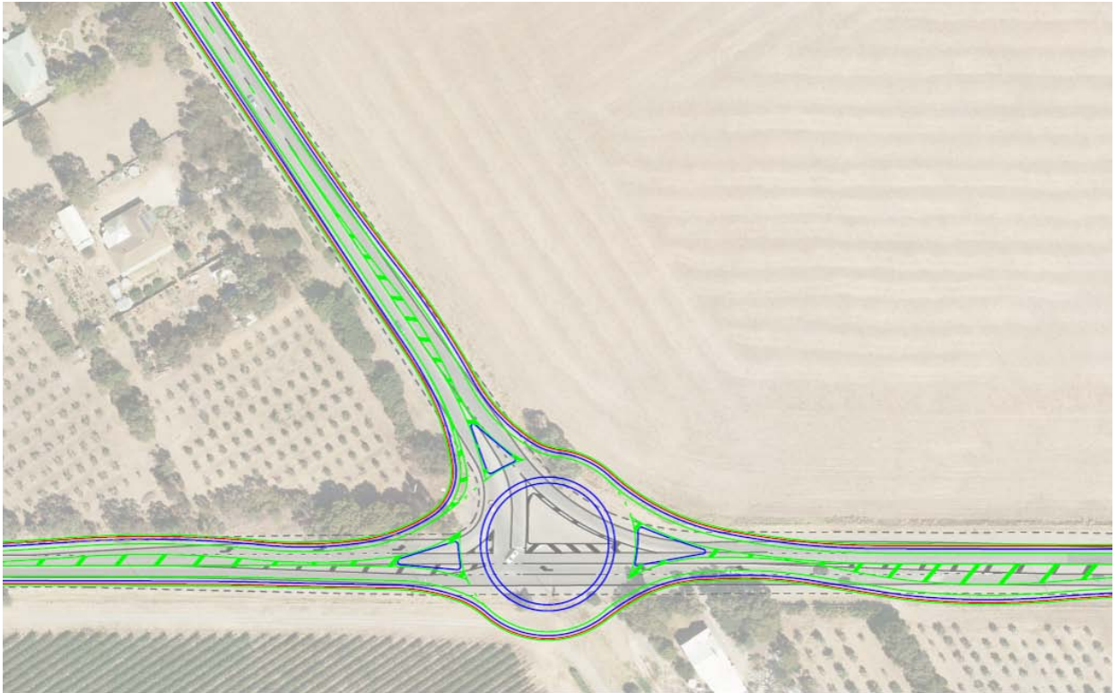
Figure 6-22: Proposed Upgrades for Aldinga Beach Road Intersection
