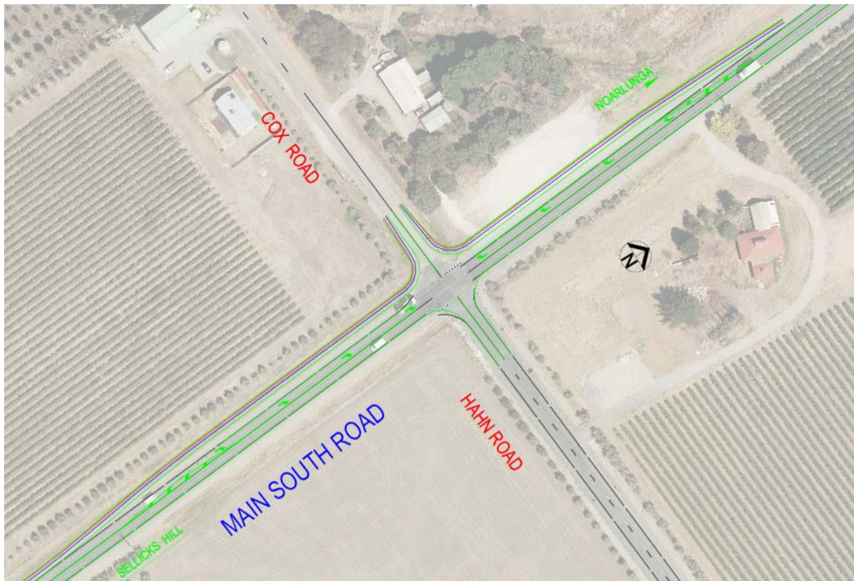
Figure 6-26: Proposed Upgrades for Hahn Road / Cox Road Intersection: – Separated Right Turn Lanes
