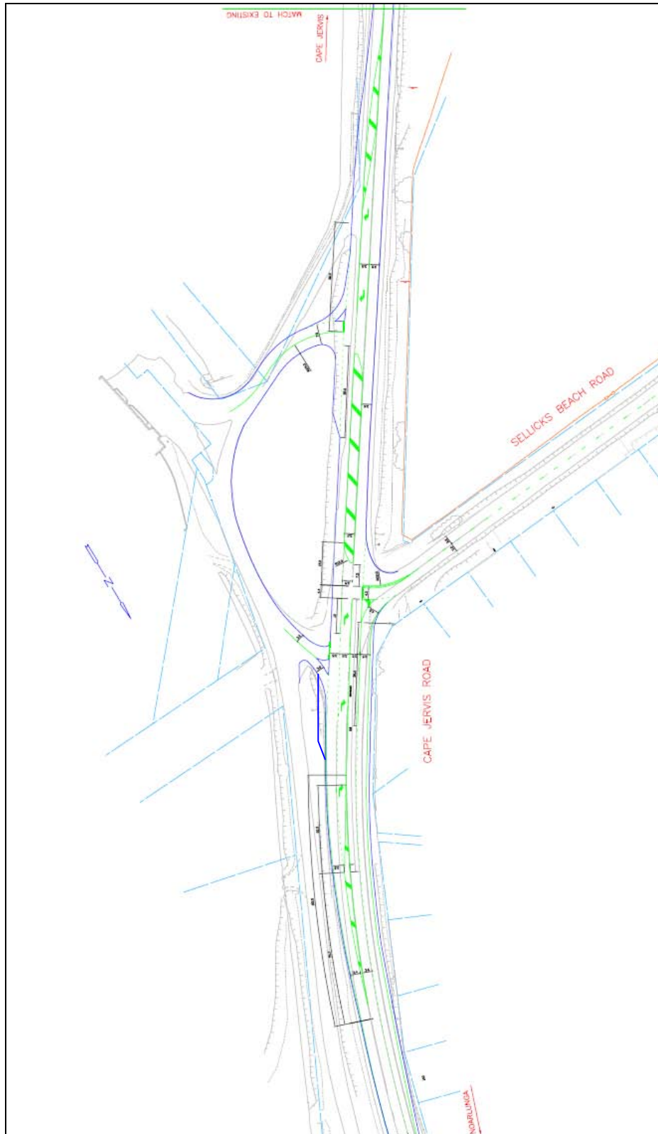
Figure 6-31: Proposed Upgrade for Sellicks Beach Road / Old Sellicks Hill Road Intersection: Realignment of Approaches and Improved Turning Facilities
