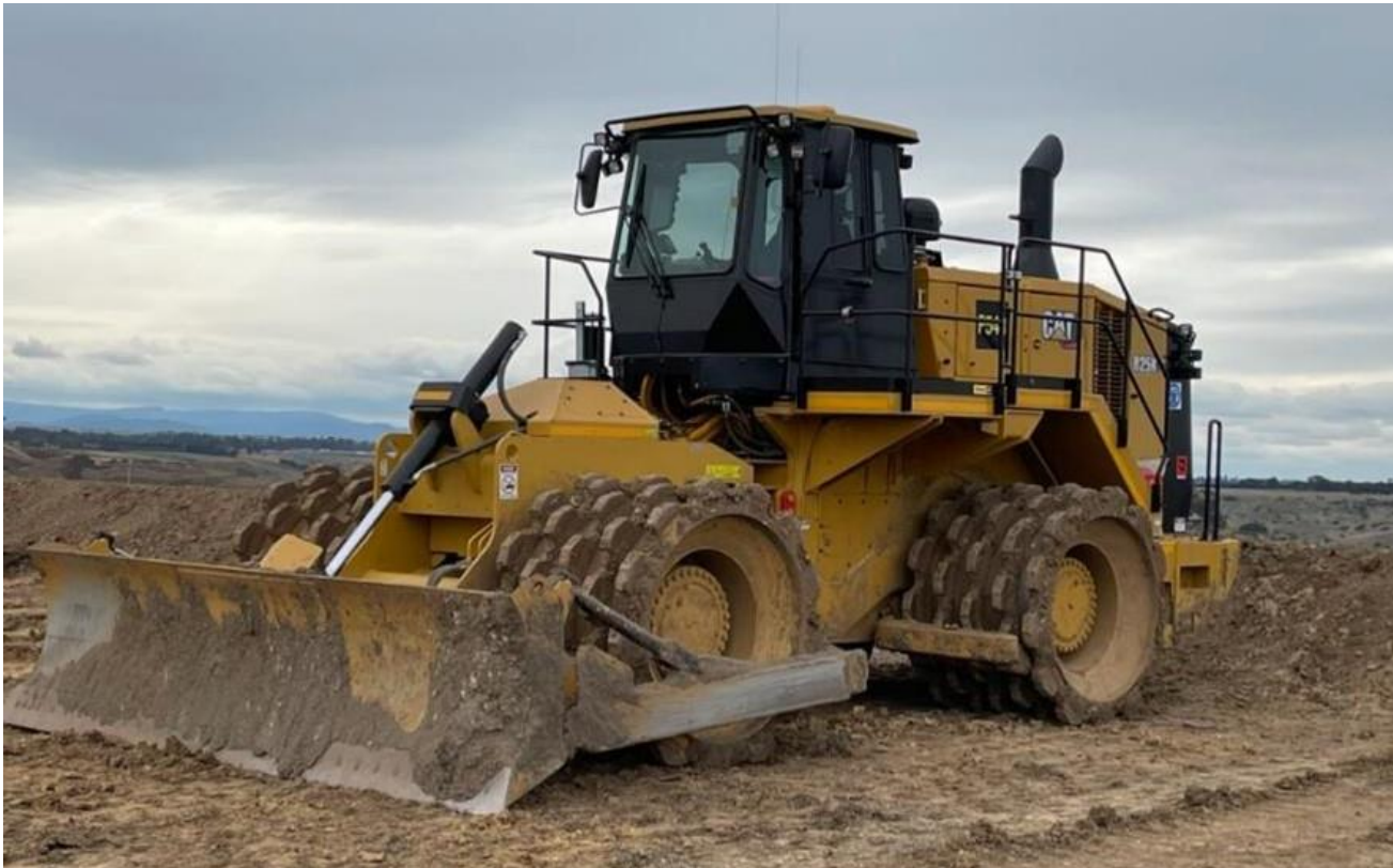
Figure 16: Example of an 'off-road' compactor used in the spoil placement area
