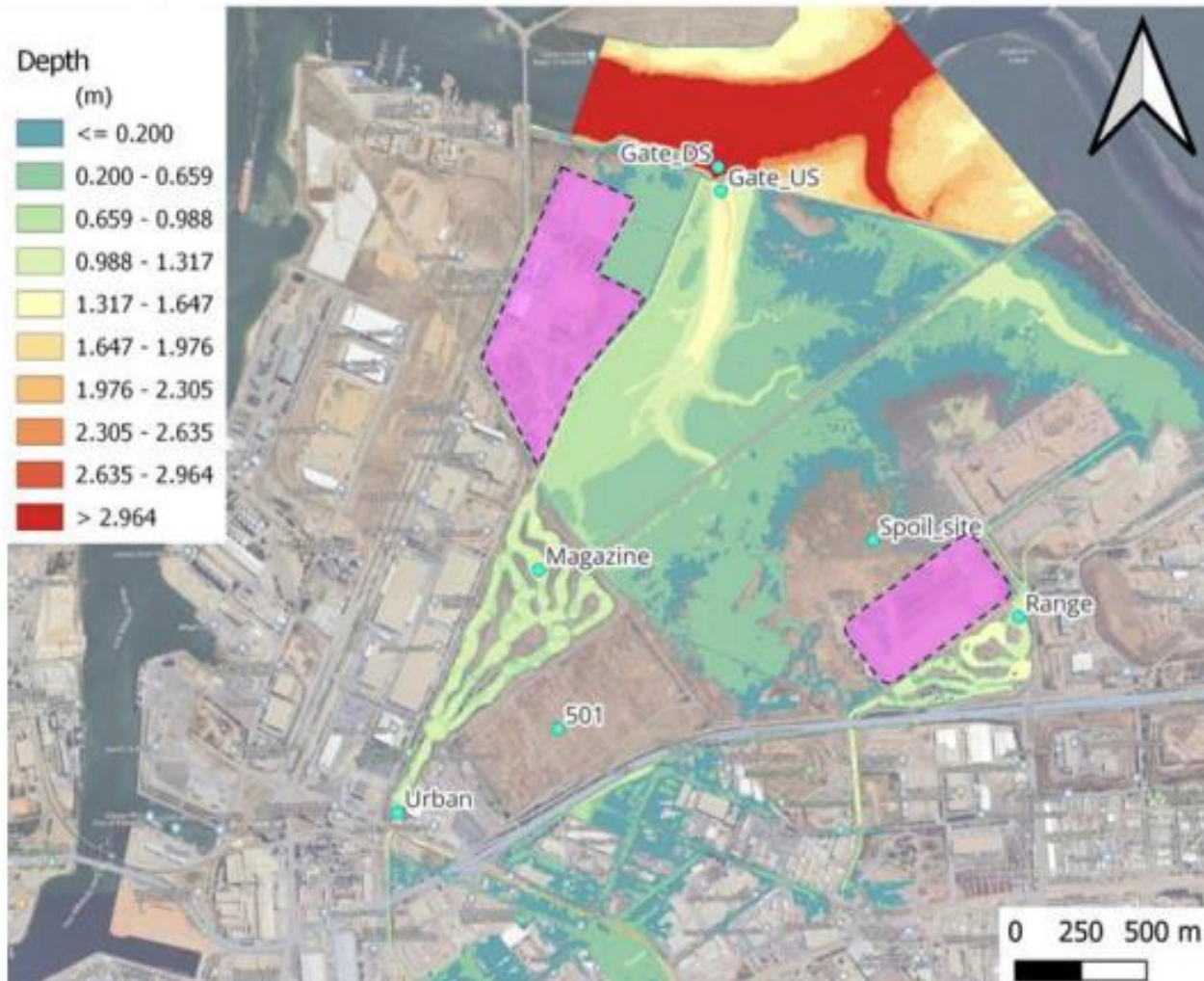
Figure 9: 1% AEP depth with MHWS and climate change with 1% AEP tidal tailwater under existing conditions
