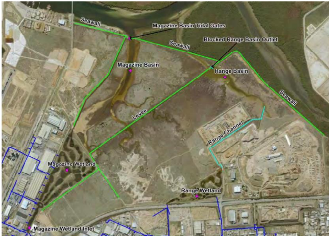
Figure 8: Gillman Basin System Overview 3
