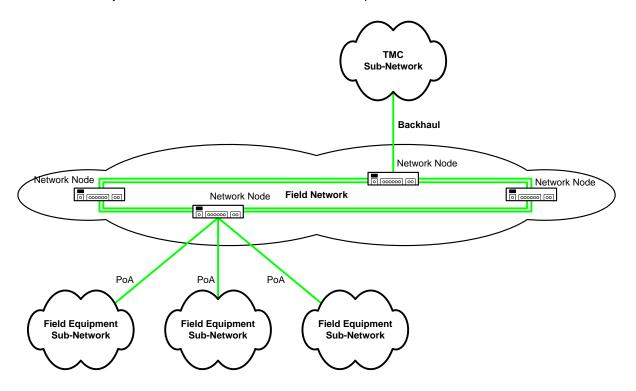
Figure 1 - ITS Network Architecture
