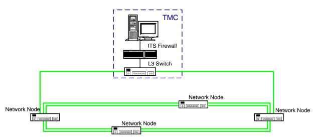
Figure 2: Redundant Fibre Ring Concept
