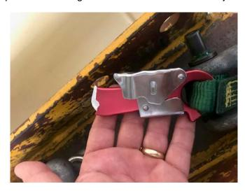
Users are reminded of the manufacturers recommendations for safe use and advice given in AS/NZS 1891.4:2009 Industrial Fall-Arrest Systems and Devices - Selection Use and Maintenance which advises against <u>back-hooking/chocking</u> as an unsafe practice.
