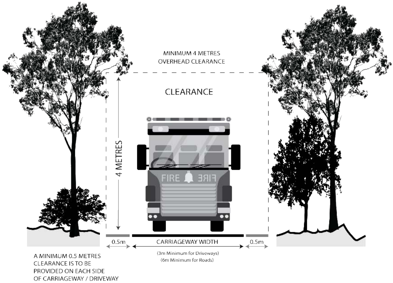
Figure 1 - Overhead and Side Clearances
