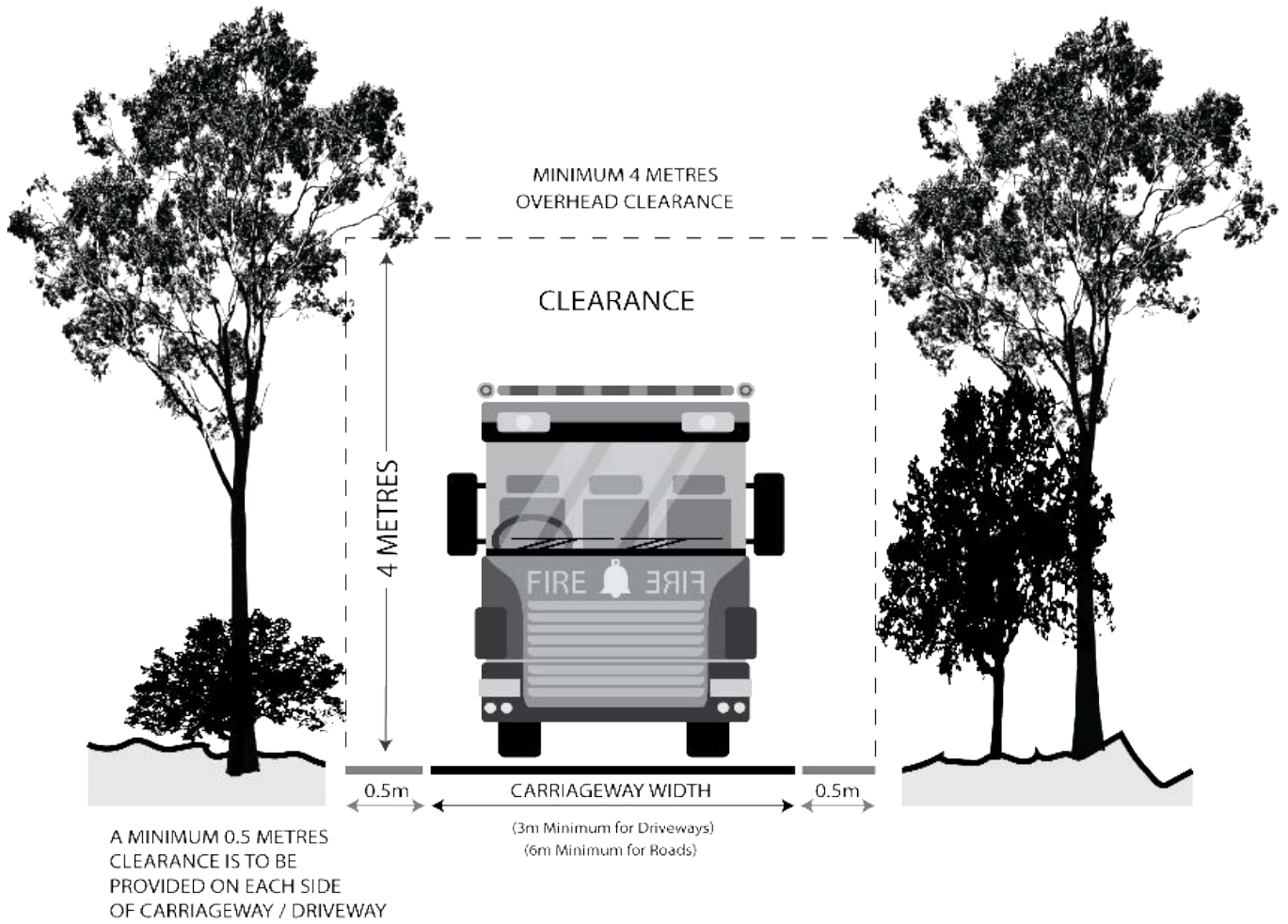
Figure 1 - Overhead and Side Clearances
