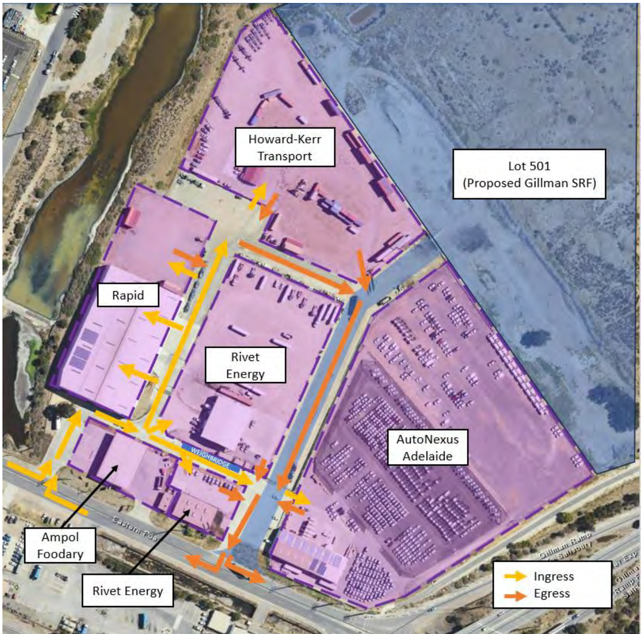
Figure 2-2 Existing Eastern Parade Business Access Arrangement (Basemap source: LocationSA)
