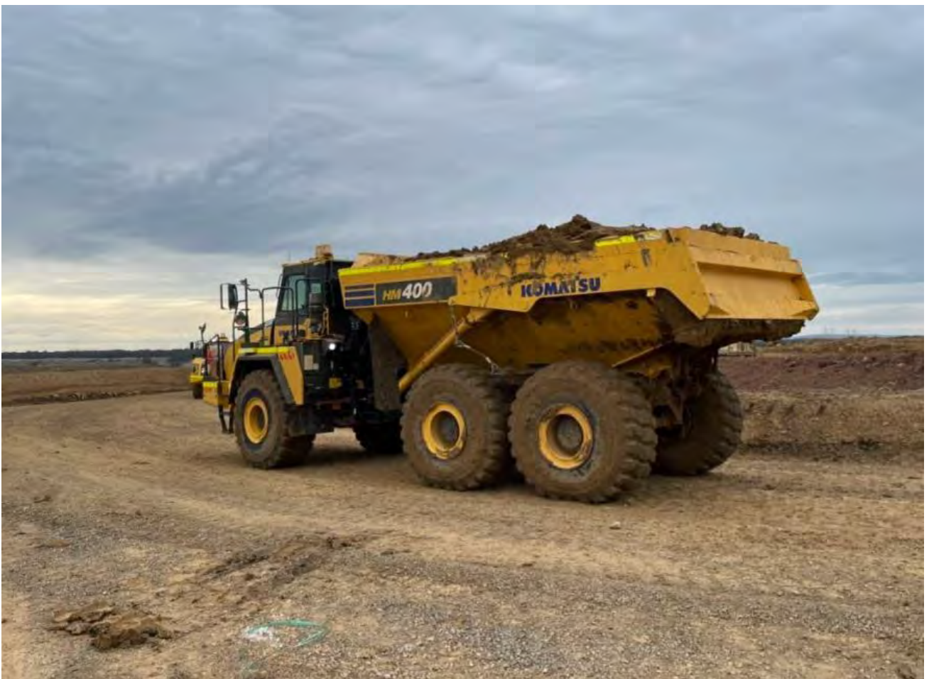
Figure 3: An example of an 'off-road' articulated dump truck or 'moxy'
