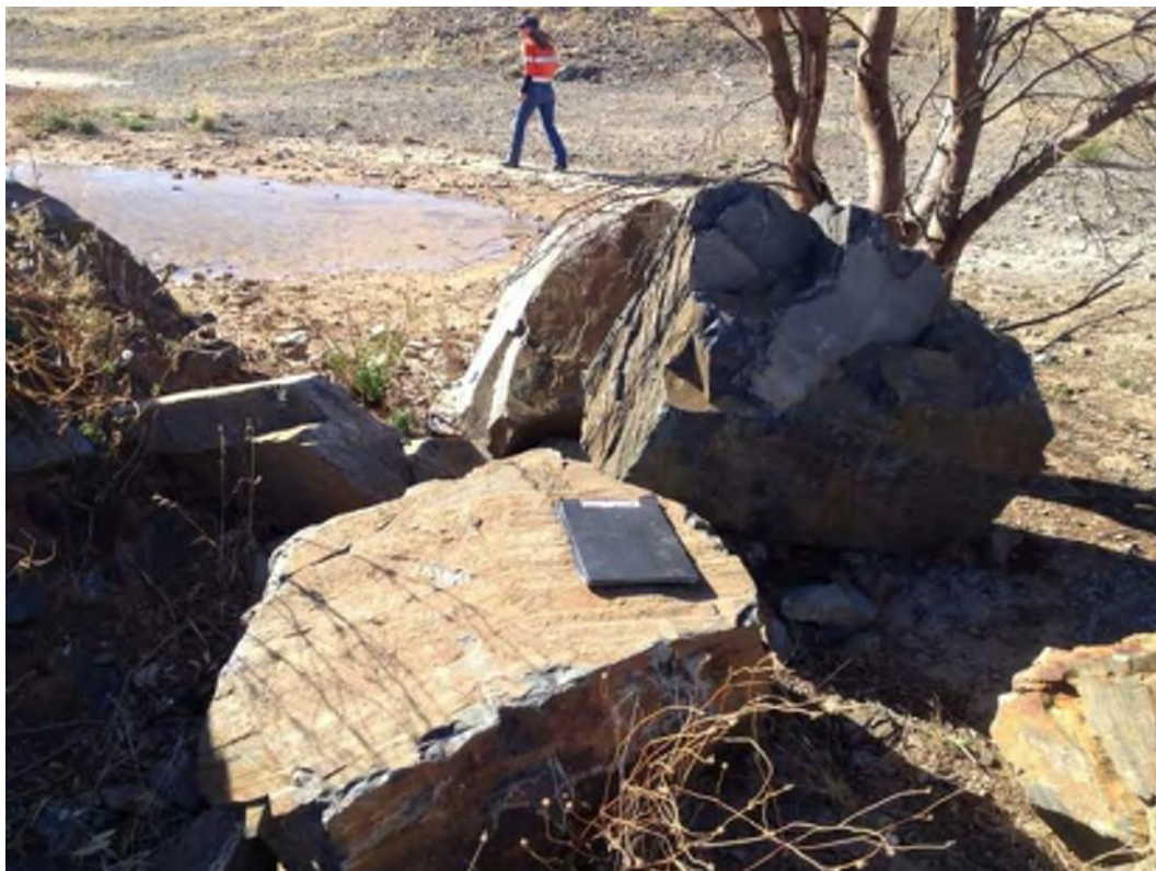
Figure 10 Photograph of borrow pit in Yerelina siltstone/sandstone
