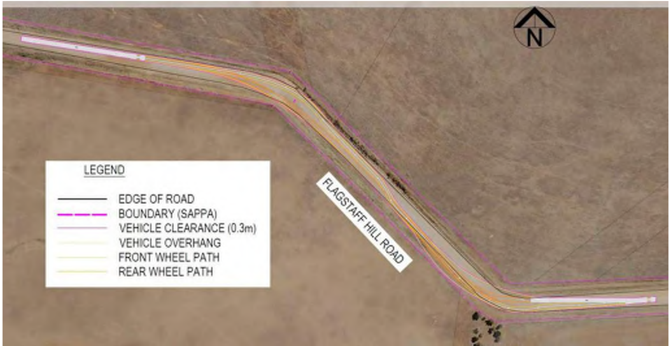
Figure 13: Vehicle navigating the bends on Flagstaff Hill Road
