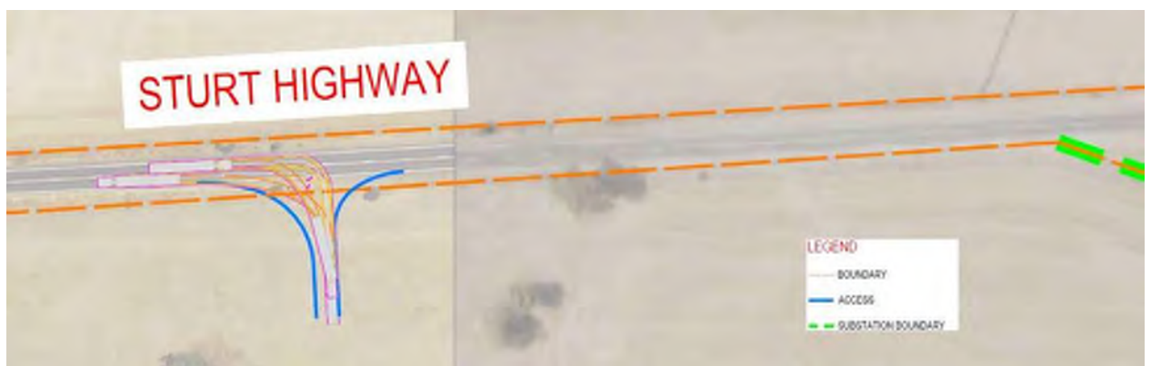
Figure 19: A 25.0 m articulated low loader vehicle accessing the terminal substation site
