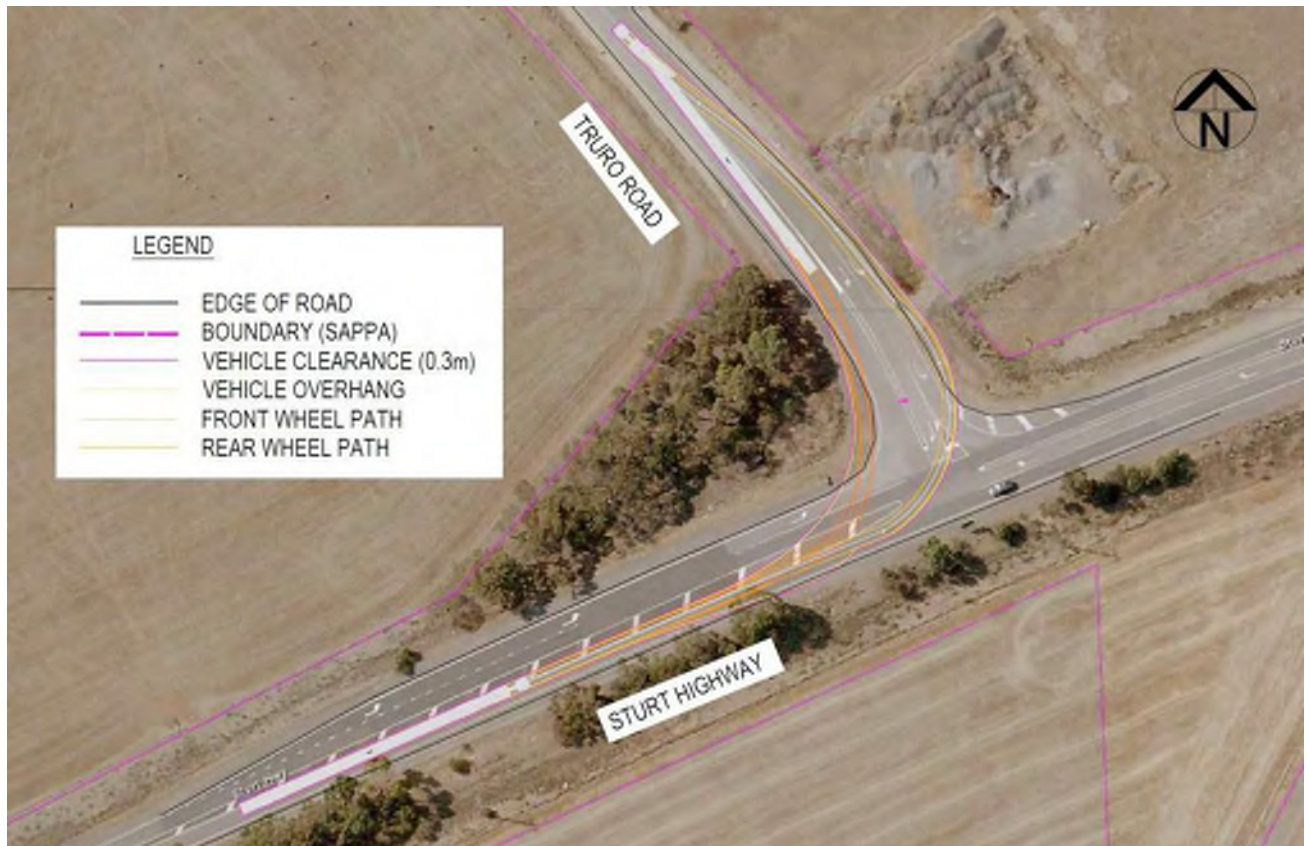
Figure 10: Vehicle navigating the Sturt Highway/Truro Road intersection
