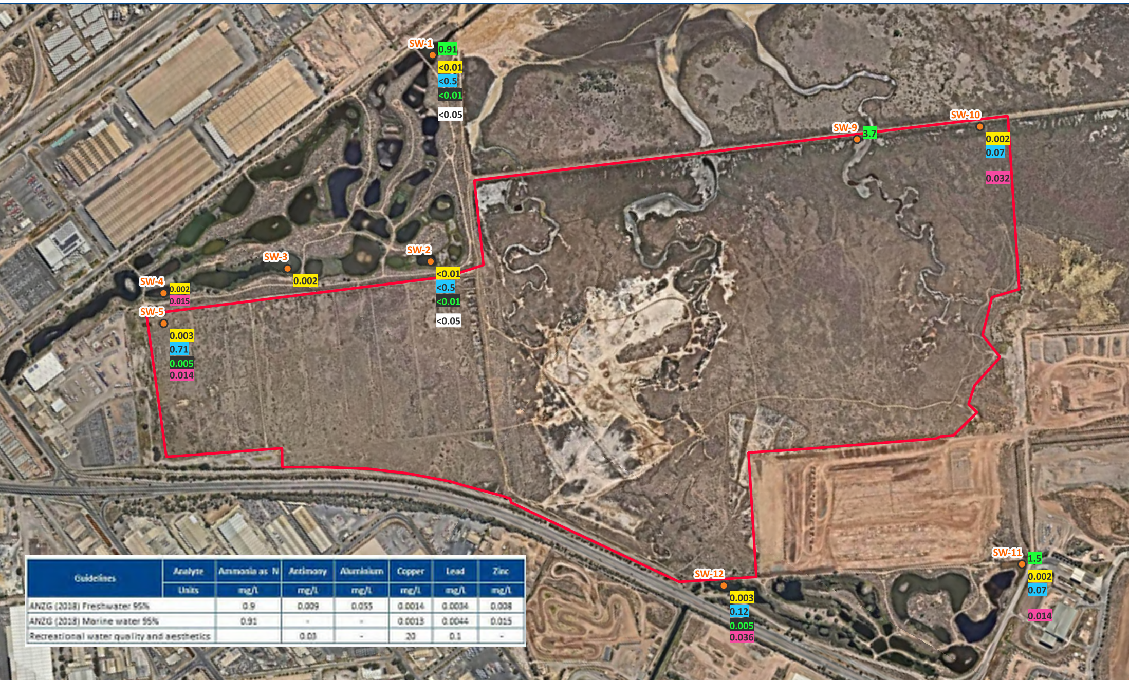
Figure A20: Surface Water Exceedances Ammonia, Copper, Aluminium, Lead, Zinc and Antimony
