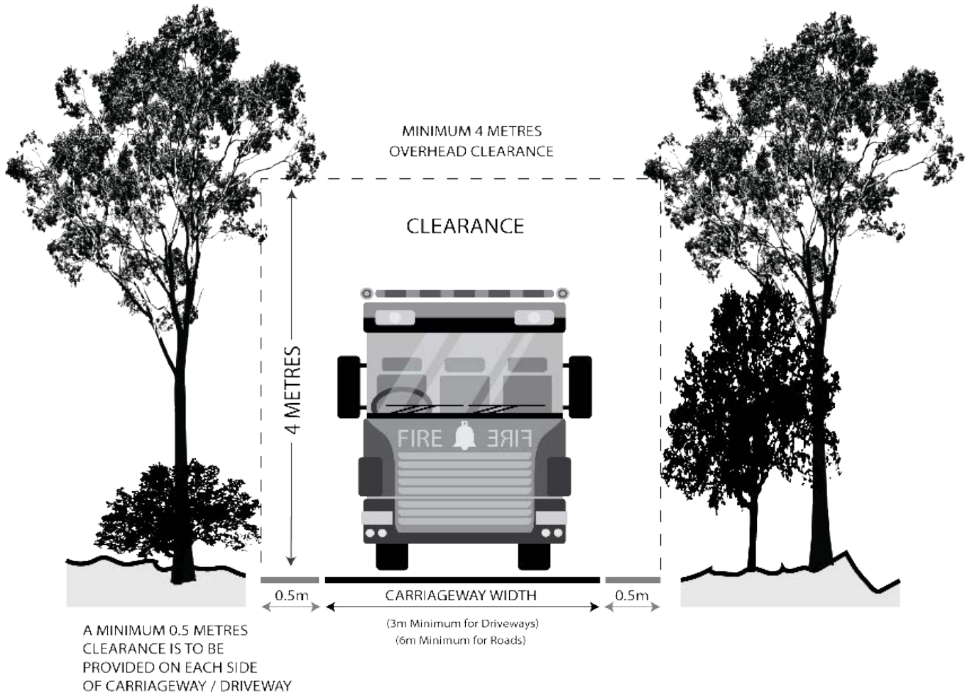
Figure 1 - Overhead and Side Clearances
