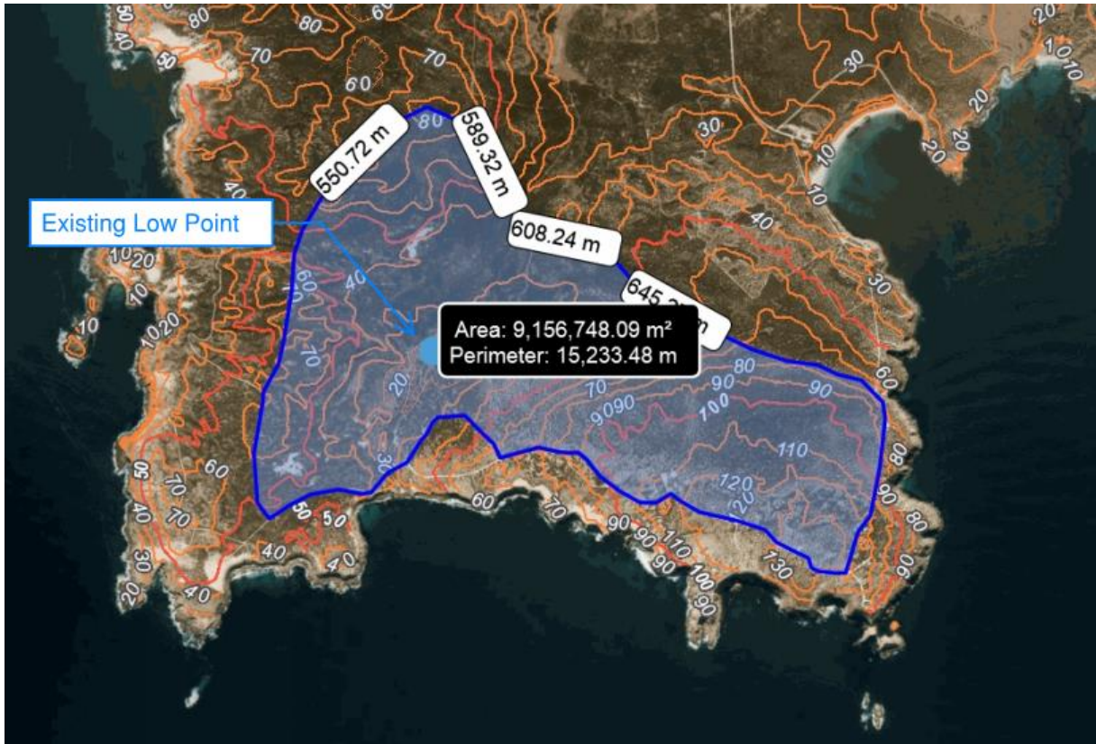
Figure 2.2 - General Site Contours and Catchment Area
