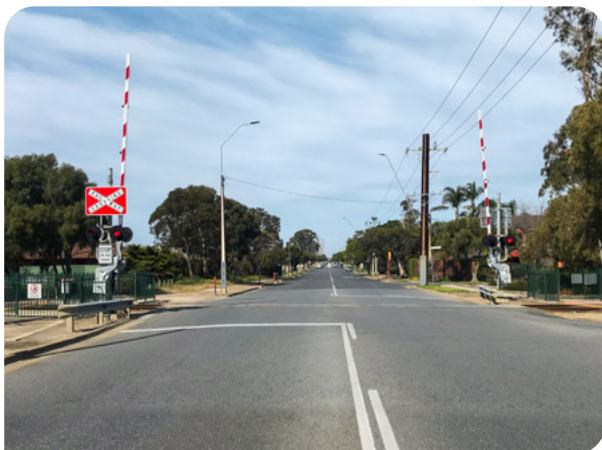
Figure 1. Example of an active level crossing – boom gates with flashing lights
