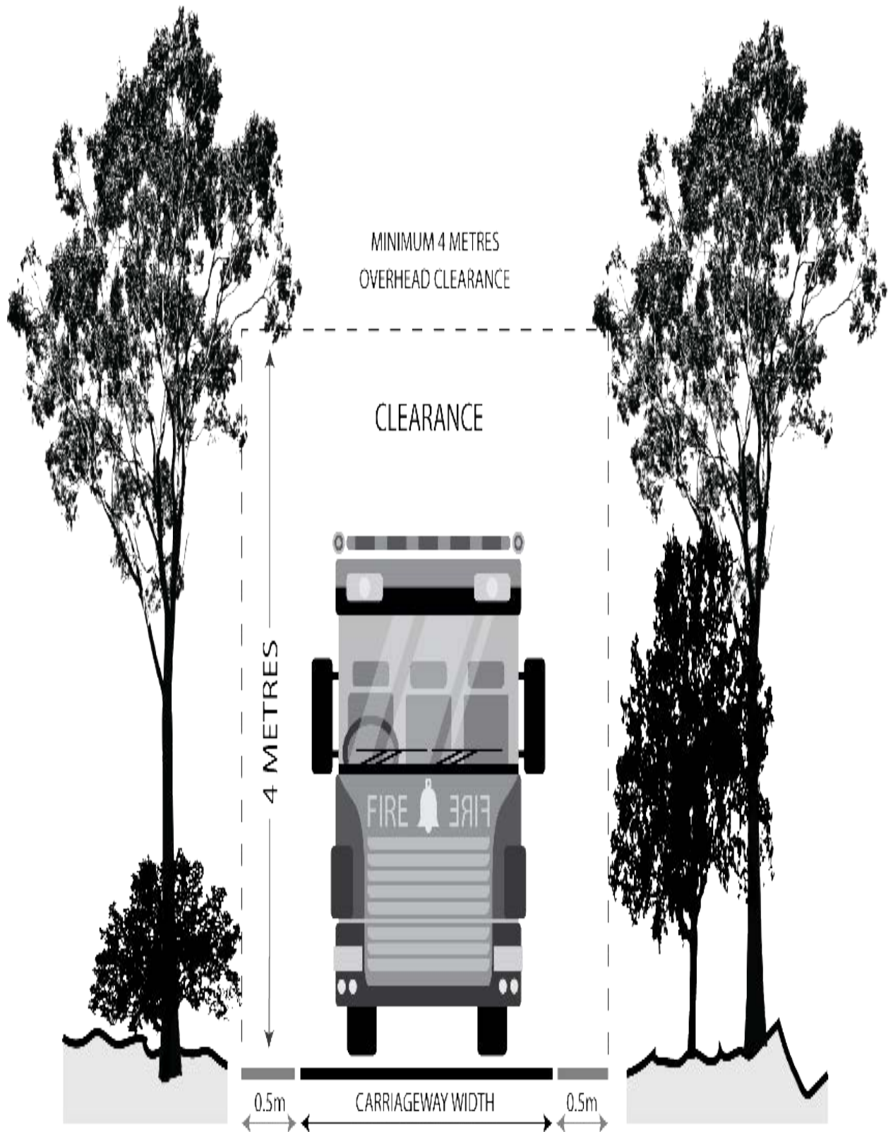
Figure 2 - Overhead and Side Clearances
