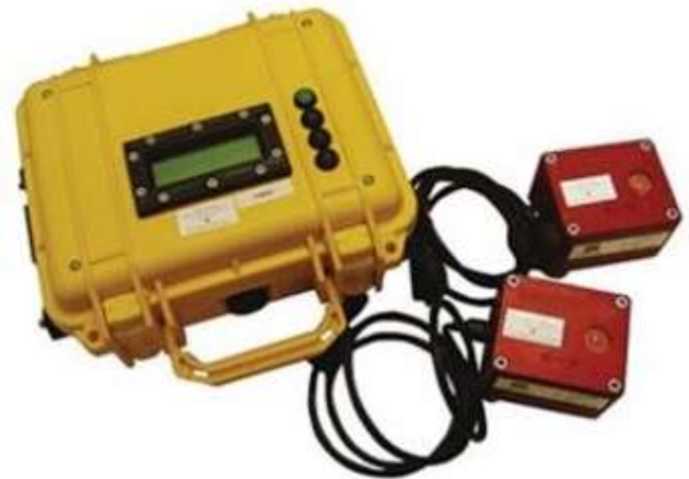
Vibration monitoring device.
