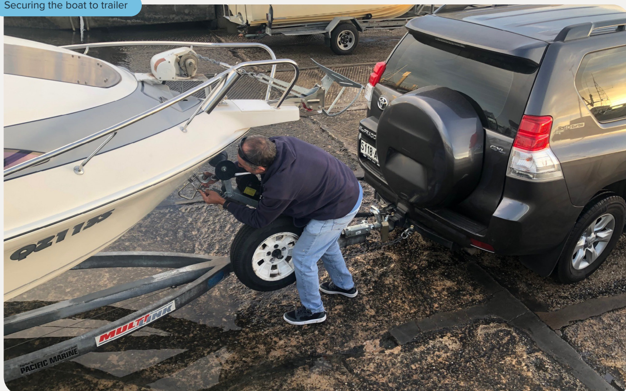
Figure 12: An example of safely securing a boat to depart a facility
