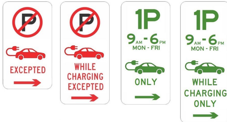
Figure 9.3 Examples of parking control signs showing use of electric-powered vehicle symbol and electric powered vehicle charging symbols
