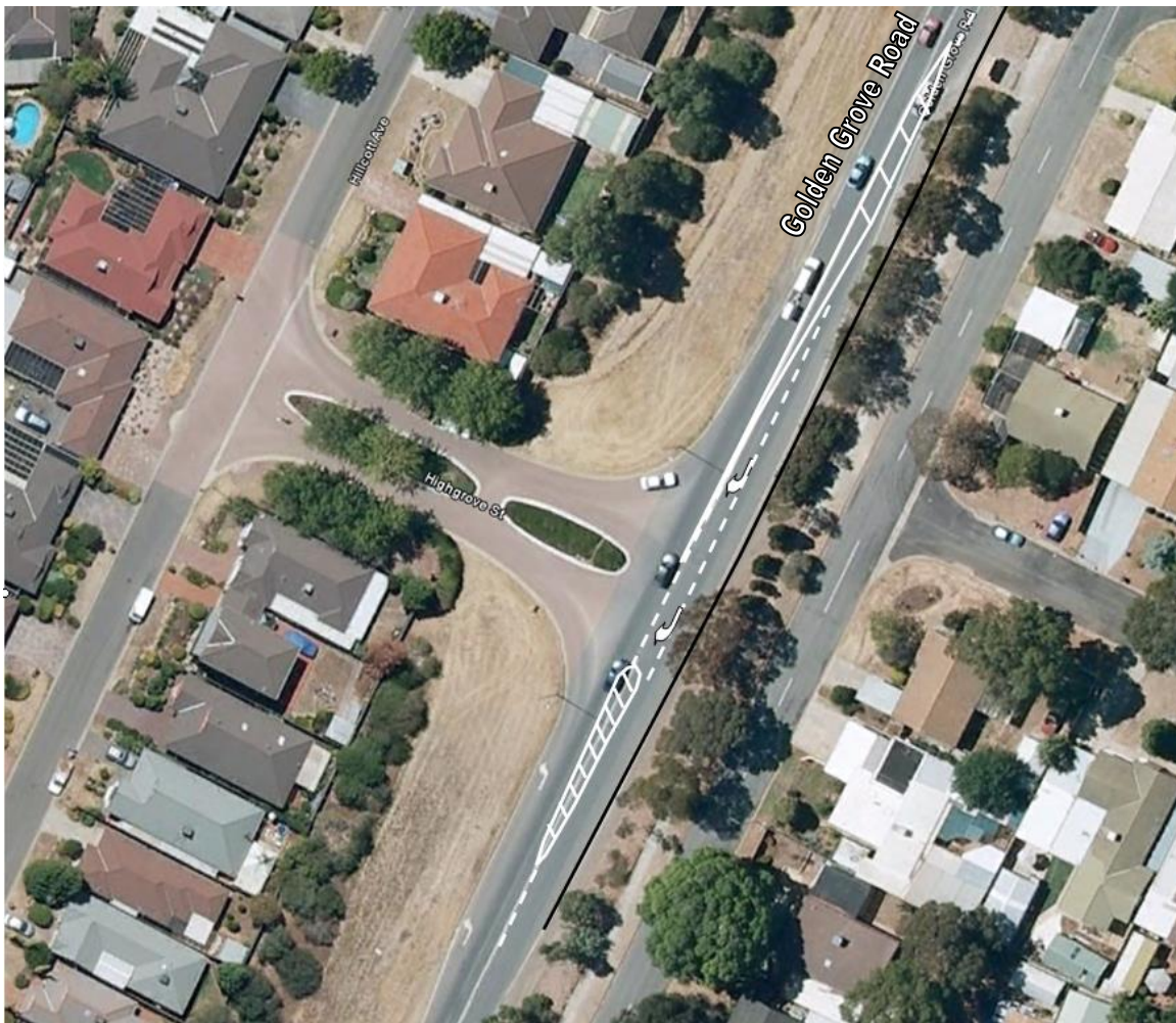
Figure 7.13: Current plan for Golden Grove Rd / Highgrove Street Intersection (channelised right turn lane)
