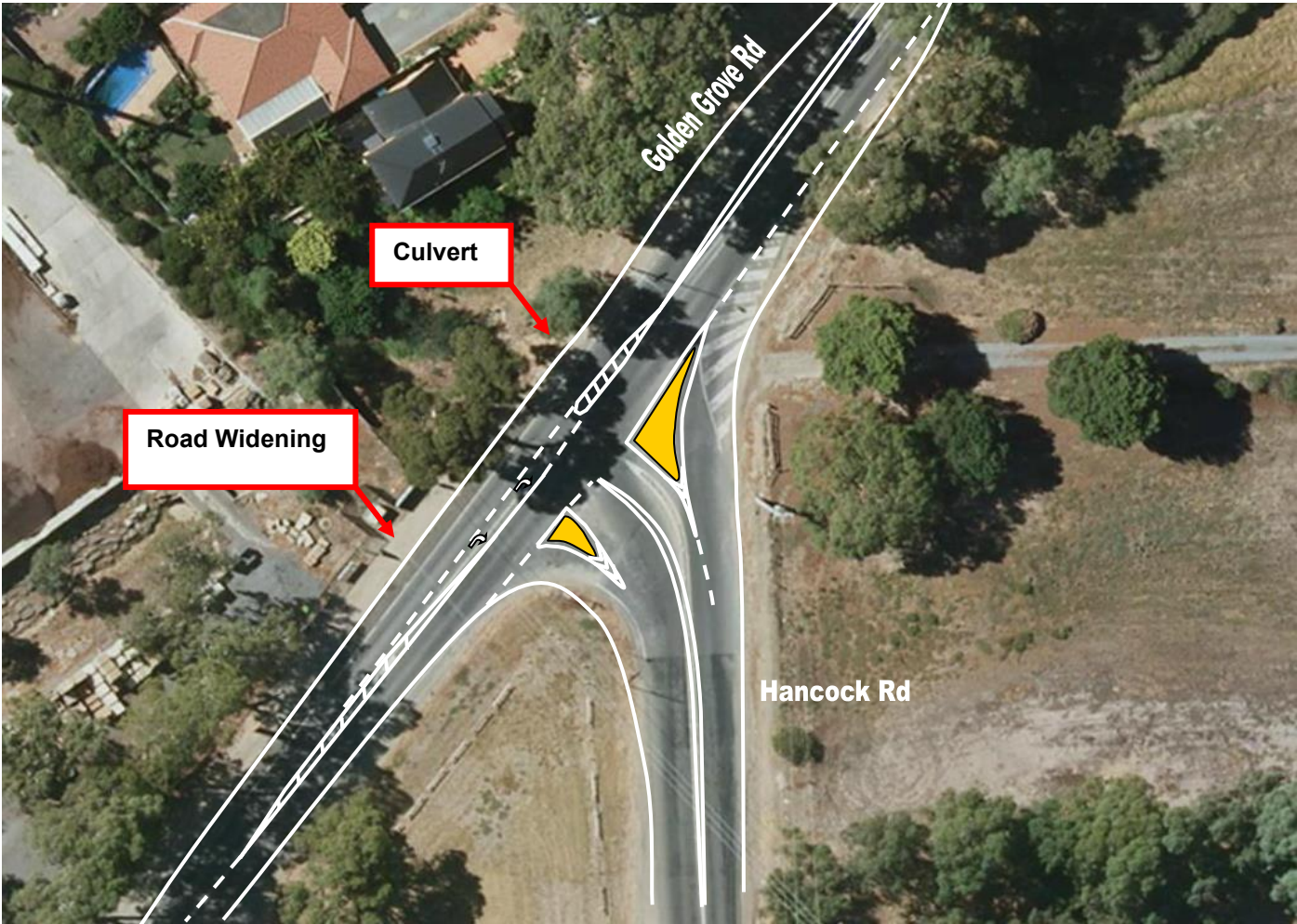
Figure 7.7: Channelised right turn lane with left turn deceleration lane concept design for Golden Grove Rd / Hancock Rd Intersection
