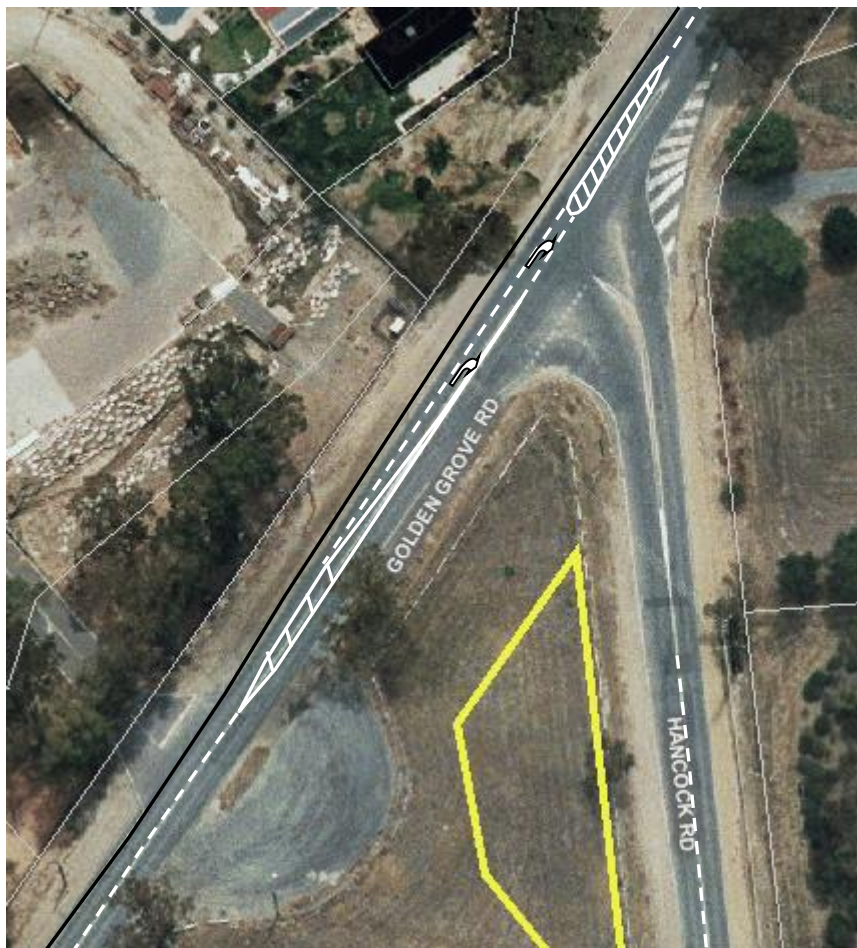
Figure 7.6: Current plan for Golden Grove Rd / Hancock Rd Intersection (channelised right turn lane)
