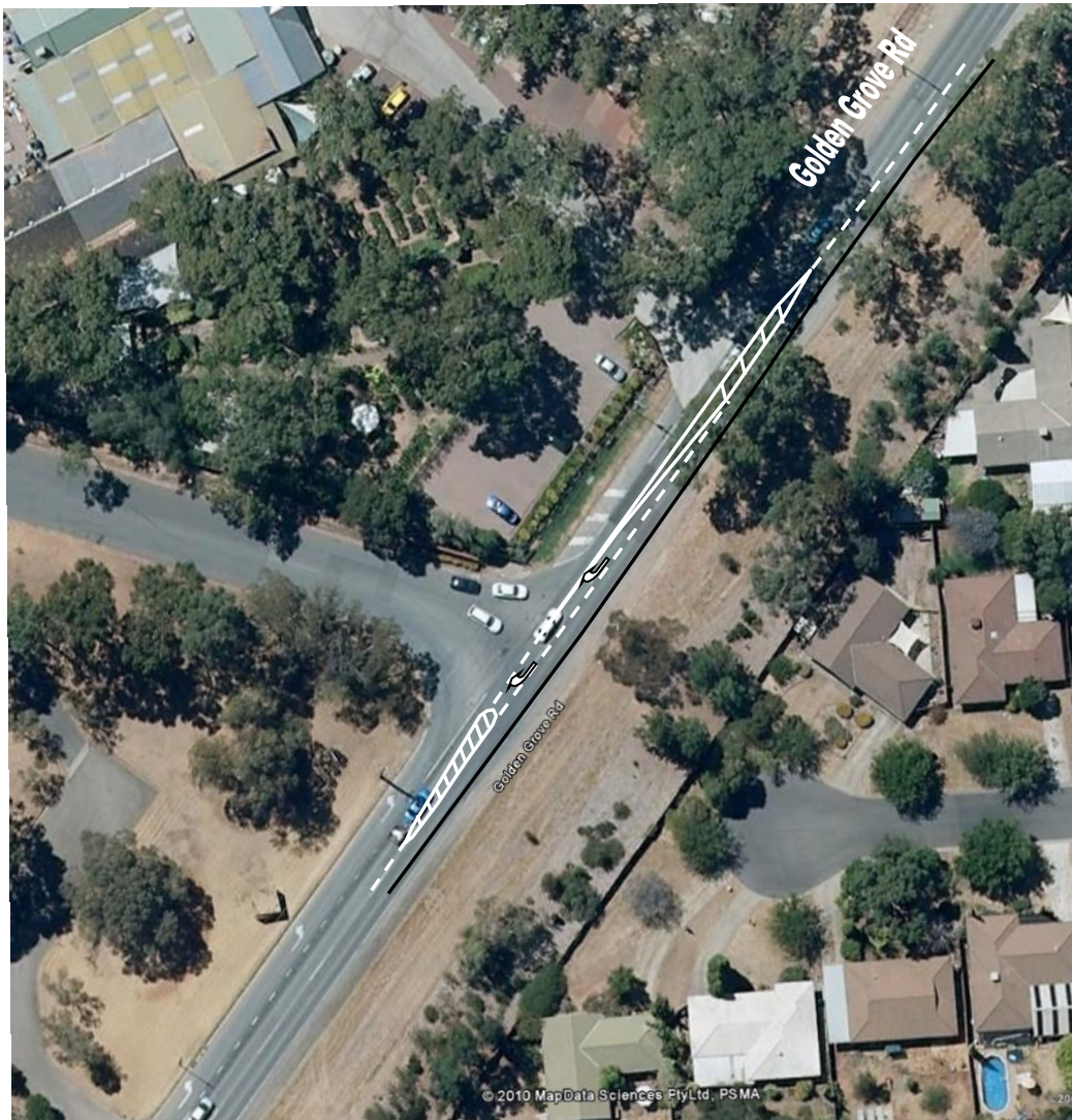
Figure 7.9: Current plan for Golden Grove Rd / Einstein Drive Intersection (channelised right turn lane)
