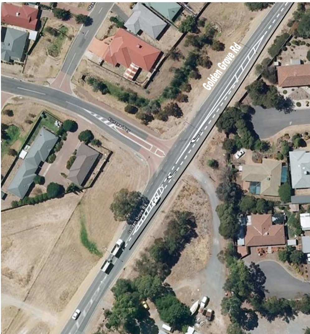
Figure 7.10: Current plan for Golden Grove Rd / Kunzea Way Intersection (channelised right turn lane)
