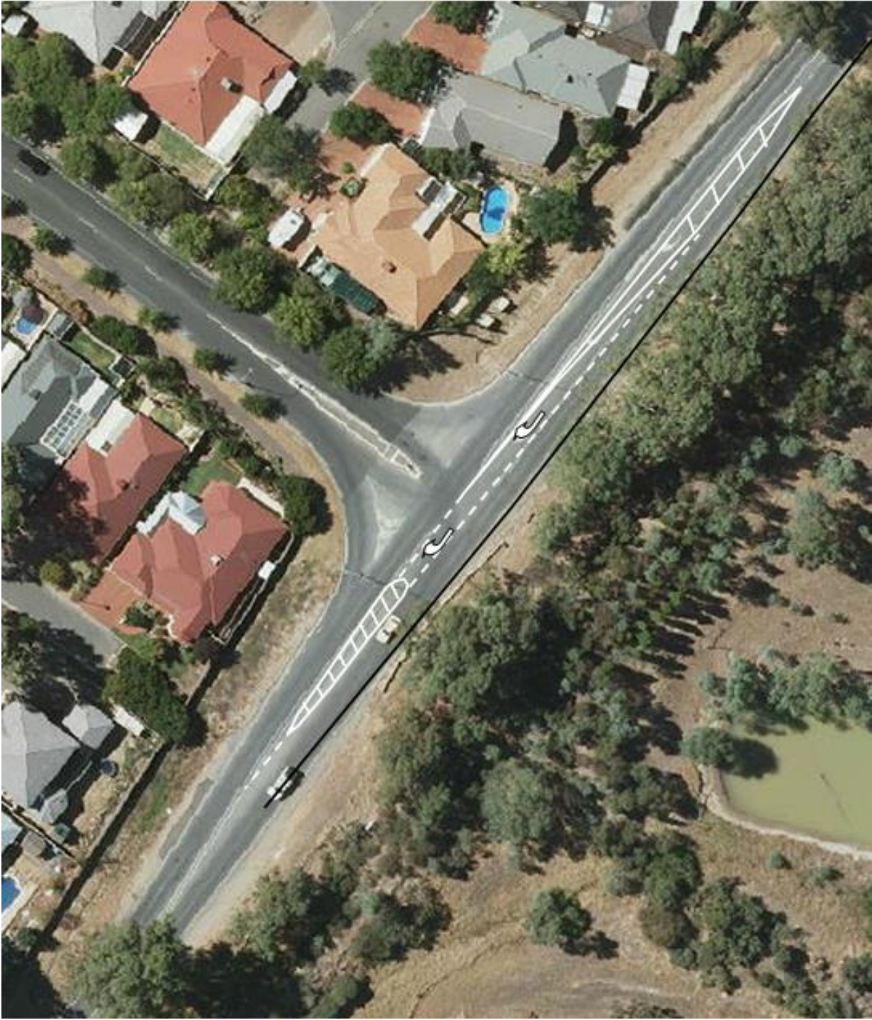
Figure 7.5: Conventional Channelised Right Turn Lane
