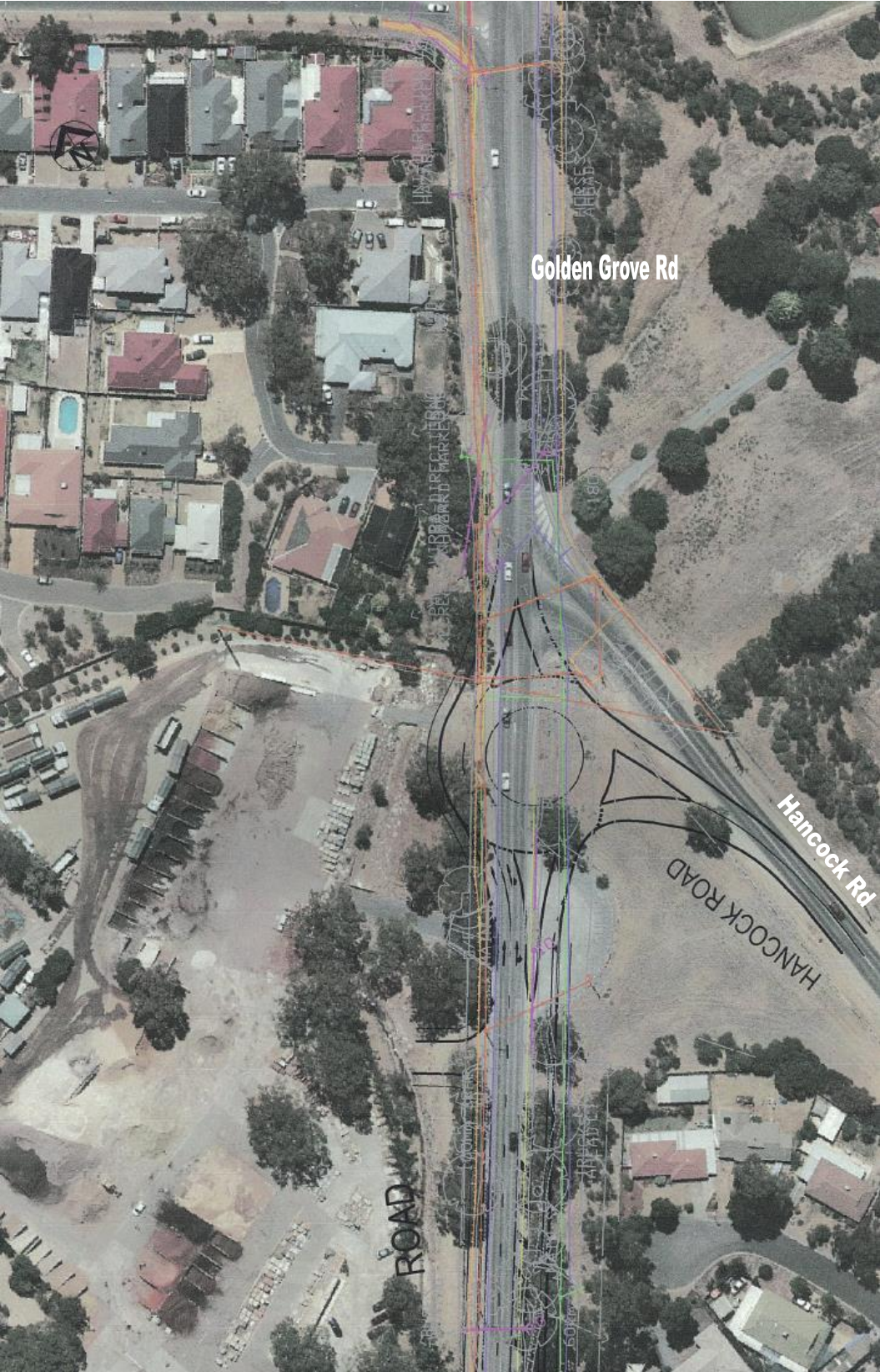
Figure 7.8: Roundabout Concept Design for Golden Grove Rd / Hancock Rd Intersection
