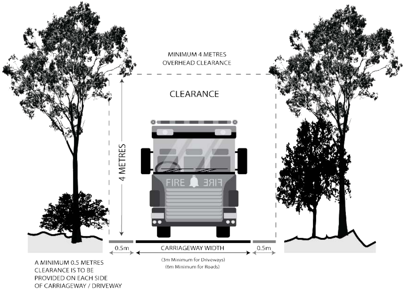
Figure 1 - Overhead and Side Clearances
