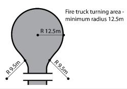
Figure 4 - 'T' or 'Y' Shaped Turning Head
