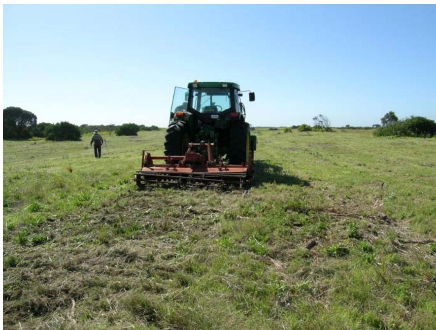
Clearance of grass cover by rotary hoe
